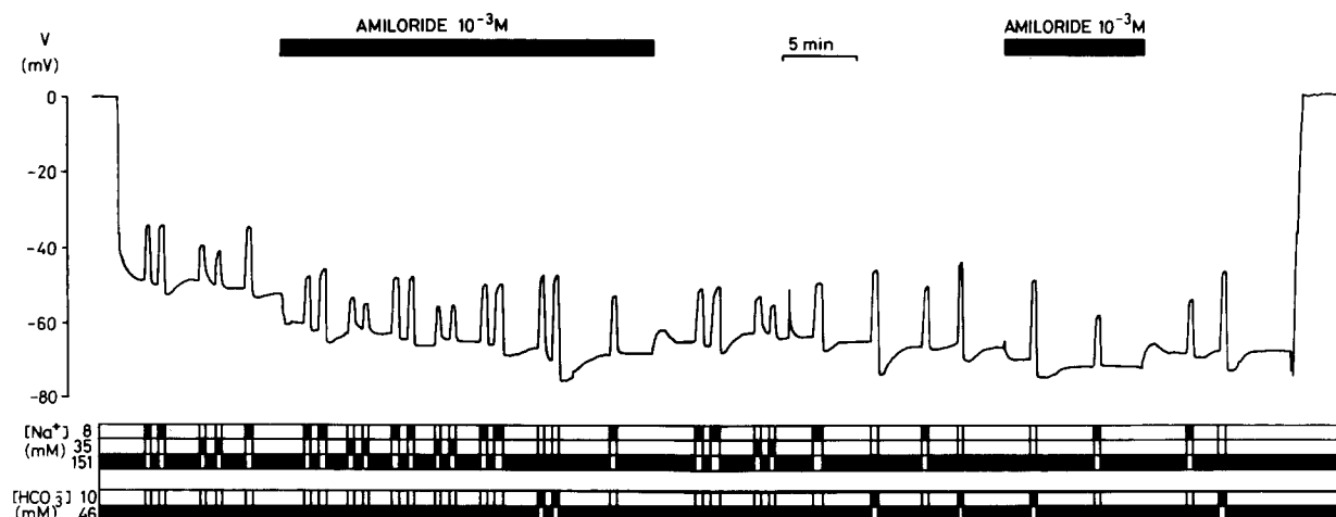
Fig. 9. Effect of amiloride ( 10^{-3} M) on the membrane potential and the voltage responses to changes in [Na^+] and [HCO_3^-] . The medium bathing the cells was replaced in short periods of 10 sec to solutions containing less sodium or bicarbonate. Note that there are no obvious differences of the reactions in the absence or presence of amiloride. Similar results were obtained with 5 other cells of 2 different strains. (Used solutions: 1, 3, 14, 16.)
